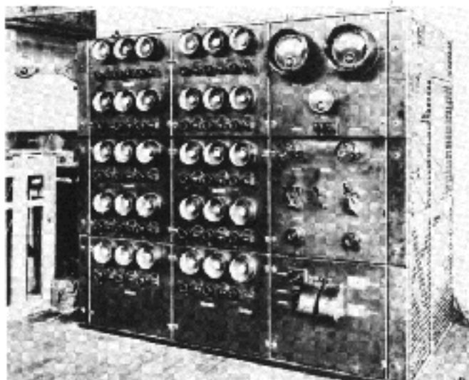
Fig. 8-10. Bank of thirty Type P Pilotrons used to modulate a 200-kilo-watt Alexanderson alternator in 1918.
